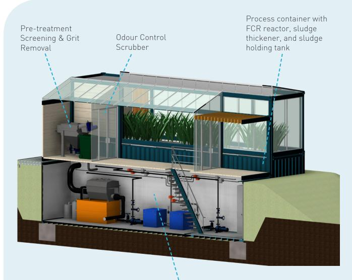
Mechanical container with mechanical, rotating equipment, electrical/controls equipment, and operator workstation
